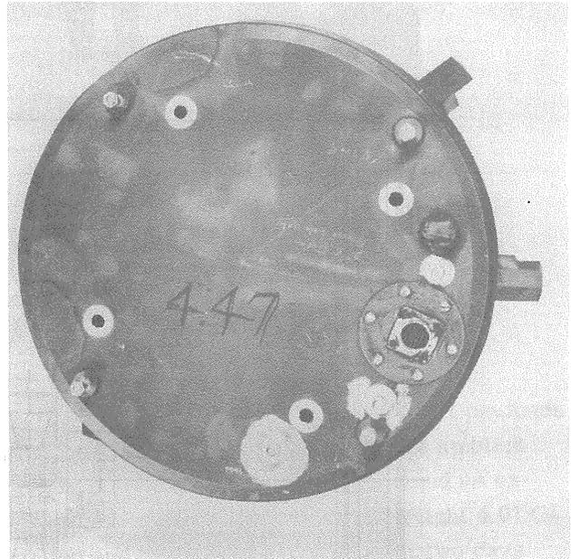
(a) Top view of parachute extension bulkhead.
