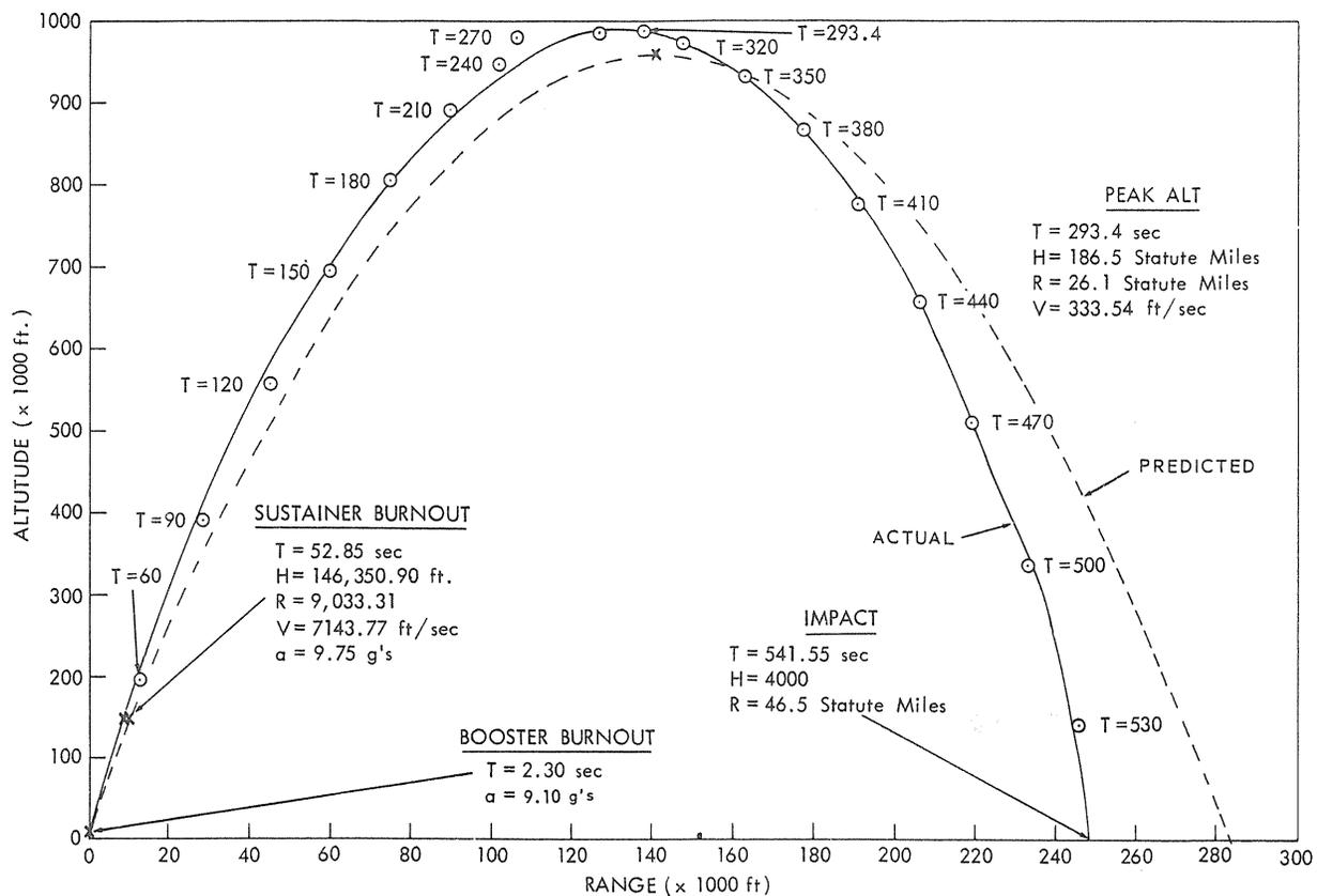
Figure 20 - Flight 4.30 GG - altitude vs. range.
