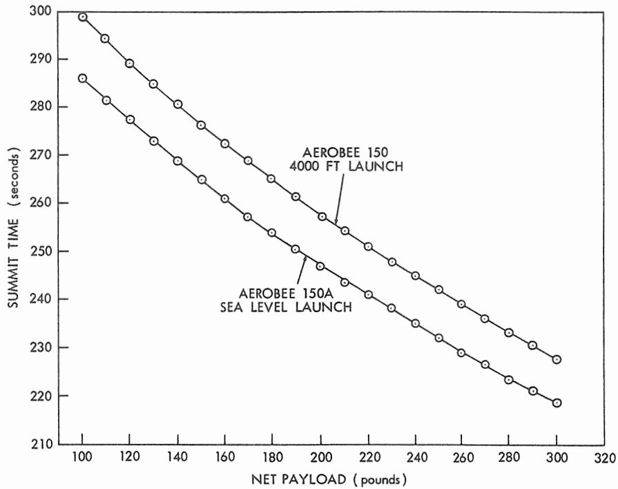
Figure A5 - Summit time versus net payload for Aerobee 150 and 150A sounding rockets with ogival nose cones and a  $QE = 87^\circ$ .
