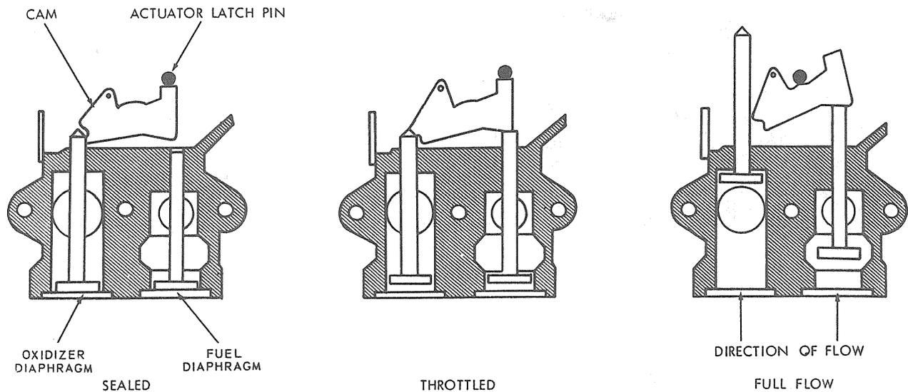
(b) Positions of propellant start valve.
