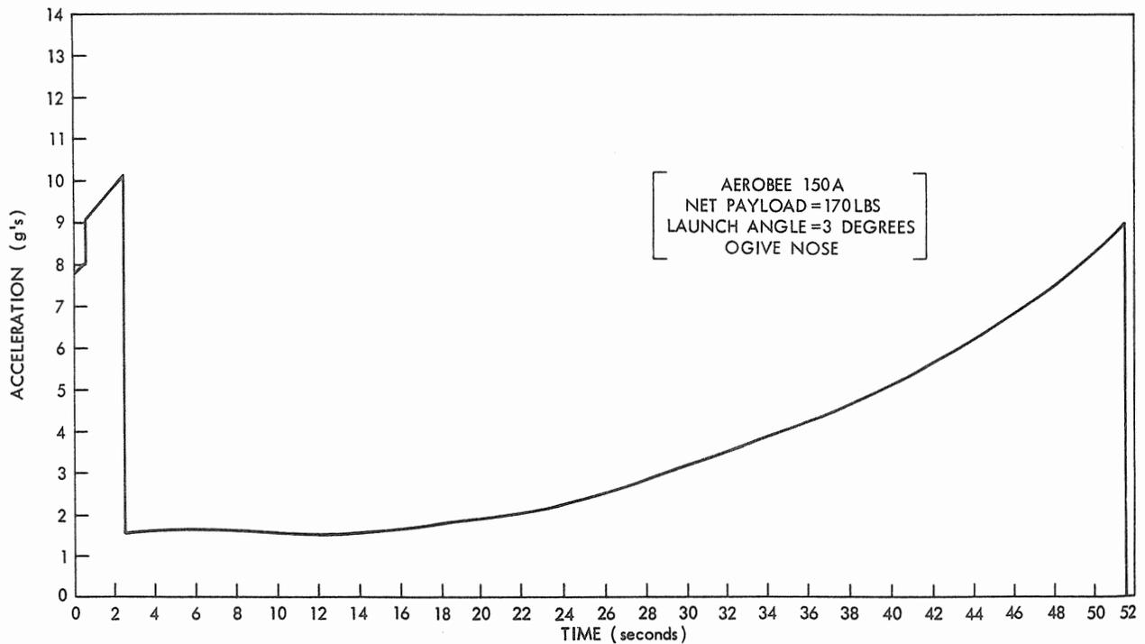
Figure A6 - Acceleration versus time for Aerobee 150A (typical).
