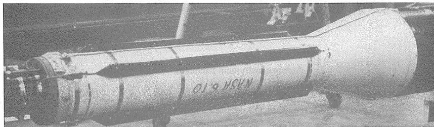
Figure 32c - Aerobee 300A, third stage motor with DOVAP transducers and antennas.
