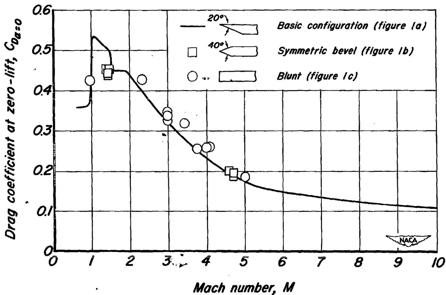
Figure 17. - Effect of fin leading-edge shape on total drag.
